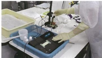
6. 脱塩液に含まれる塩化物イオン濃度の測定 Measurement of the chloride ion concentration contained in the desalination liquid
