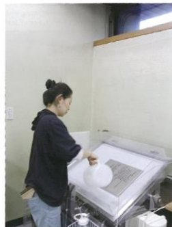
6. 漉きばめ機を使った作業 Repair process using a leaf casting machine
